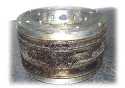
Shown is a seal that failed due to lack of continuous clean, dry buffer gas. John Crane reports that such a deficiency causes a majority of the seal failures the company sees during compressor refurbishments. Photo courtesy of John Crane Inc.
