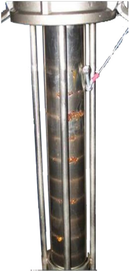
CONTAMINATION CAPTURED BY THE MAGNETIC FILTER ELEMENT
