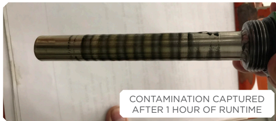
TRANSMISSION RUN STAND WITH OEI INLINE MAGNETIC FILTER SCRUBBER
