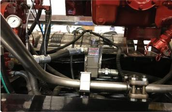
Lube oil filtration for the np1000 NOV triplex required improvement to the existing depth media filtration provided. OEI's willingness to work with us to create a filtration product that included depth media filter required by our customer base and a magnetic filter element allowed us to create a single device that does both things for the customer. This product is inside - out flow – prefiltration by the Magnetic Filter Element and secondary filtration by the depth media element.
