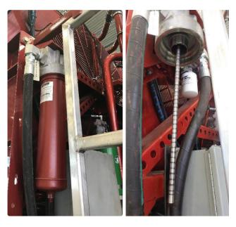
Deployed in all hydraulic triplex high-pressure pumping applications. All scrubbers have low pressure drop so they work well with highly viscous oils without causing wear damage for the lube oil pump that lubricates the triplex device.
