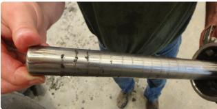
Diesel fuel injectors, because of the extremely high operating pressures up to 30,000 PSI, will become scored if 5-micron wear particle cleanliness isn't maintained. Once scored or washed out from fine debris moving at high fluid velocities, filtration efficiency drops and emissions increase.
