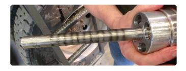
This filter is working in conjunction with existing depth media filtration – because of the magnetic filtration, the conventional filtration is expected to last longer because the Magnetic Filter Element removes the fine contamination before hitting the depth media.
