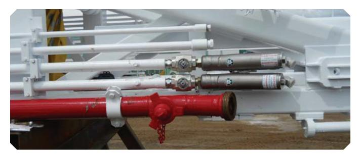
Precison Drilling has installed two of these high pressure magnetic filter scrubbers on 28 of their first generation Super Single Top Drive rigs. Precision is also using various other OEI magnetic filters on their Super Single rigs in the return filter housings of their open loop hydraulics.
