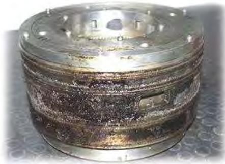
*Shown is a seal that failed due to lack of continuous clean, dry buffer gas. John Crane reports that such a deficiency causes a majority of the seal failures the company sees during compressor refurbishments. Photo courtesy of John Crane Inc.*
