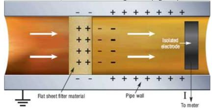
In pipeline flow, the streaming current will be discharged back to the pipe walls, reservoir or component surfaces, and the discharge rate is controlled by the characteristics of the fluid and its additives. This charge relaxation is described by the equations below:
